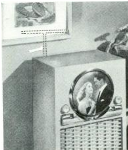
Indoor antennas need not be exposed to view.
