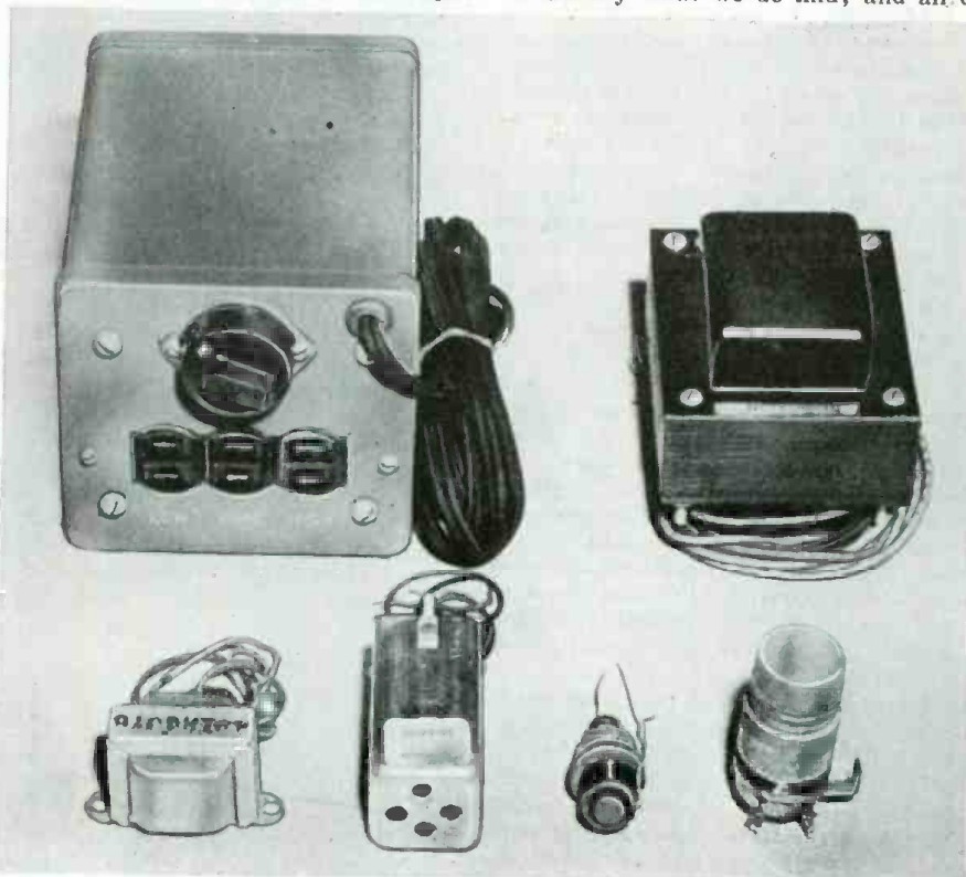
Some of the many types of transformers used in radios. Rear we have an isolation and a power transformer. Front, an output, an i.f., iron-core r.f. and an antenna transformer.
