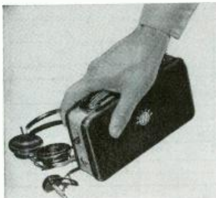
Nuclear "Sniffer" uses vibrator power supply.
